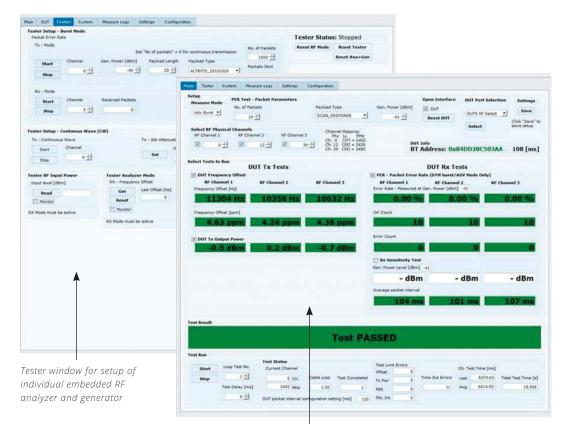
Main window for configuration and execution of RF measurements
