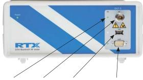
Status LEDs RF to DUT USB to DUT UART 2&4 wire to DUT
